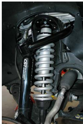
COIL OVER'S INSTALLED
