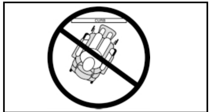
Figure 3. Incorrect Curb Approach
