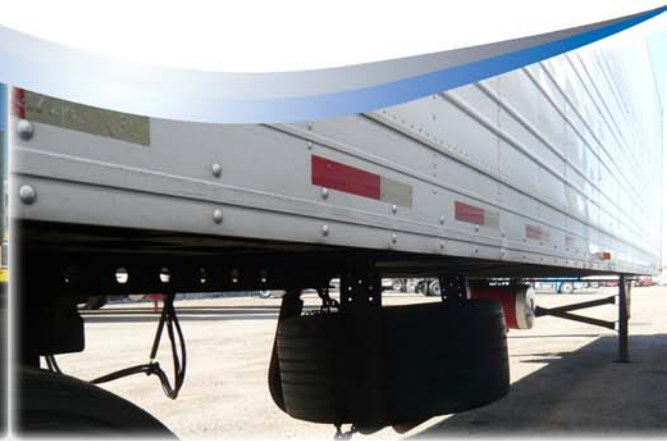
Traditional bucket tire mounts do not allow tire access with side skirts
