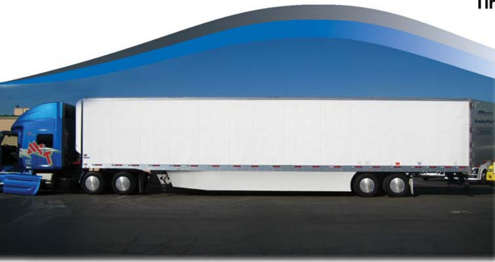
SuperSpare™ for Trailers allows under-trailer storage of super single or regular tires, with or without side skirts
