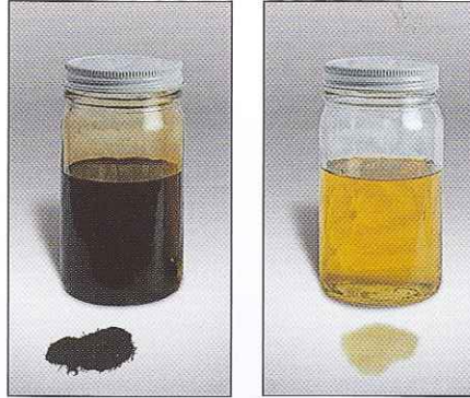
Dirty power steering fluid (left) can compromise the performance of the steering system and may even cause damage.
