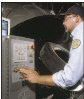
The Bandag 7400 Insight® Casing Analyzer
